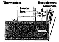
Electric dryer with back panel removed
